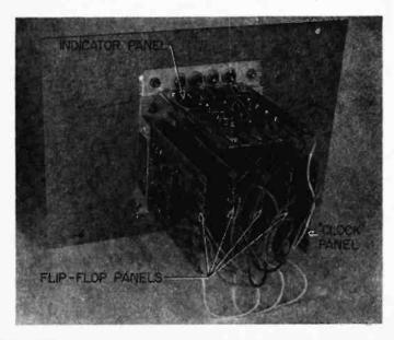
Rear view of the Digilette front panel shows all the circuit panels secured in place and interconnected. Some careful planning is necessary in order to avoid unsightly holes or marks on front panel.
