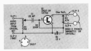
In a typical set-up, the AudiAmp (above) is connected to the phone terminals of the Knight-Kit Crystal Set 83 Y 261D.
