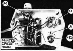
The 600-ohm resistor is unsoldered from the circuit board at the location shown.
