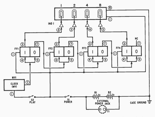
Wiring diagram for the Digilette. Logic symbols are used for the flip-flop, clock, and indicator modules to simplify the drawing and promote rapid understanding.
