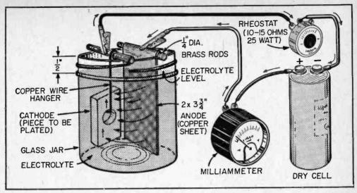
DIAGRAM SHOWS plating tank with cathode (piece being plated) suspended in electrolyte.
