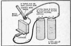
THE BRUSH-PLATING circuit diagram shown here has a cotton swab with copper wire anode connected to the positive terminal. Copper and nickel are the easiest metals to plate. Clean the cathode of all traces of oil.
