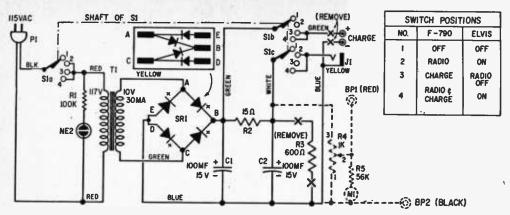
Schematic diagram for ELVIS. Dashed lines are circuit parts added to the Lafayette F-790.
