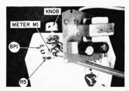
With the circuit board lifted out of the way, parts added underneath can be seen.
