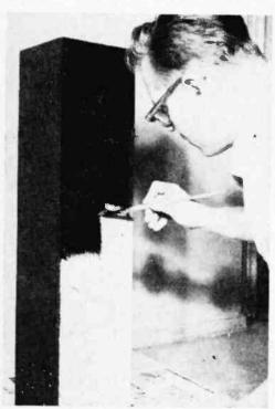
COAT the assembled column with flat, black paint. It will highlight grille cloth's coloring.
