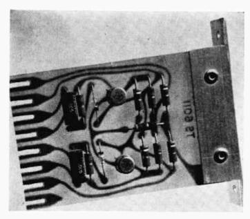
Component side view of the Tech Serv's Digibit flip-flop circuit panel. Bracket seen at right serves as common ground that connects to the positive terminal of the 12-volt DC supply.
