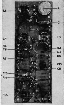
Almost all of the interconnecting wiring are on the bottom side of the circuit board. Small press-in terminals allow handy anchor and interconnection points between parts.
