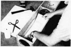
FOAM RUBBER is used as acoustical padding to line all sides of the airtight upper chamber.
