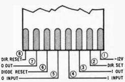
The Tech Serv Flip-Flop FF-1 (left) is a bistable multivibrator that is the basic oogic element used in the Digilette. The flip-flop is activated by a positive-going input pulse. The terminal module connections are diagrammed above.
