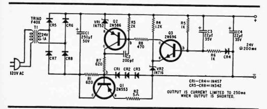
Fig. 6. Schematic diagram of 24-volt regulated power supply that powers the music adapter.
