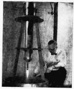
EXPERIMENTAL electric generator directs plasma past magnets in tank of liquid helium.
