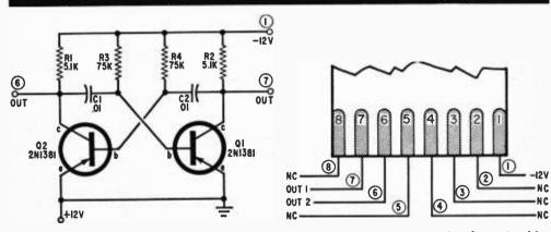
Circuit diagram of the Tech Serv Clock MV-1 (left) that operates at about 1 kc. determined by the R-C time constants of C1, C2, R3, and R4. Terminal connections shown at the right.
