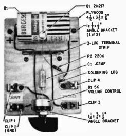
Parts needed to assemble the AudiAmp are shown above wired on a plywood chassis.
