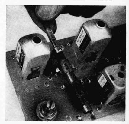
Alignment of the completed music adapter requires an audio signal generator and either an oscilloscope or an AC VTVM. There are four tunable Miller coils.
