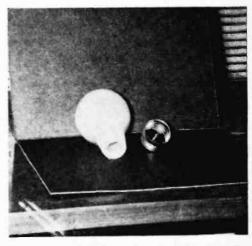
A bugger's delight is the plastic light bulb. Remove base (top) and insert tiny mike. Installed in lamp socket (below) line cord serves as audio cable. Keep switch set at on.
