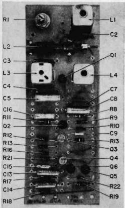
Top view of the music adapter circuit board showing the neat uncluttered arrangement of parts. Location is important. Refer to the detail circuit board drawing on page 48.
