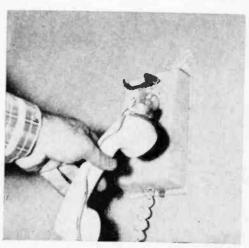
Inductive pickup lets you tape telephone conversations without connecting to wires.
