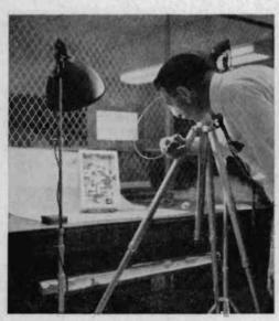
Under chassis shots require lights to be set wider apart than normal to eliminate shadows in deep corners. Check very carefully in order to prevent confusing reflections.
