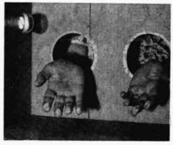
Ultraviolet lamp inside "crime detector" box spots incriminating fluorescent tell-tale smudges on thief's fingertips. Low cost Argon bulb provides adequate ultraviolet light.
