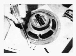
SPEAKER is mounted on 7-in. square of plywood. Screwdriver points to two solder lugs.
