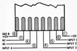
The schematic diagram for the indicator circuit is shown at left. This Tech Serv unit contains four amplifiers, each driving a lamp mounted on the front panel. When the input to any amplifier is at ground level, an appropriate lamp will light up. Drawing above shows terminal connects for the module. Lamps are General Electric type 1201.
