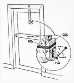
Ordinary mono or stereo cartridges can be utilized as sensitive sound pick-ups.
