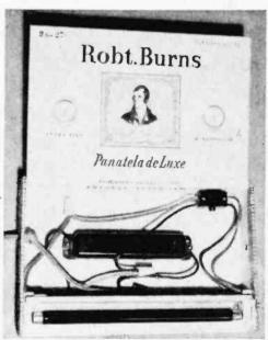
The ultraviolet lamp kit can be installed in a cigar box as shown above. Text explains construction details. Home made unit is compared to Edmund Scientific professional unit (left). The large window in the pro type unit passes long waves and the small window passes the harmful short UV light waves.
