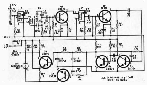
Fig. 4. Schematic diagram of the transistorized music adapter—operates on 24 volts.
