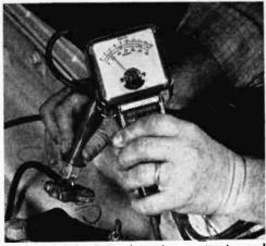
COMBINATION volt and ammeter is used to record battery voltage. Volt meter is connected in parallel with circuit being tested. Ammeter is attached in series to show draw.
