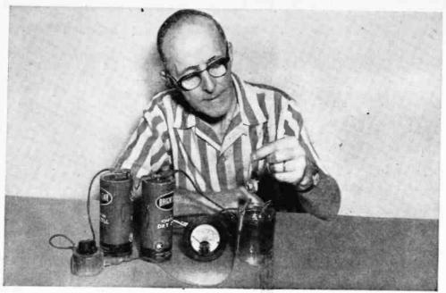
TABLE-TOP ELECTROPLATER uses dry cell batteries, rheostat, milliammeter and plating jar.
