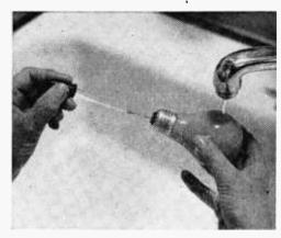
Special bulbs are prepared by alternately heating and cooling light bulbs with hot and cold tap water. See text for details.
