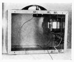
Inside view of the Digilette showing the location of power supply circuit parts.
