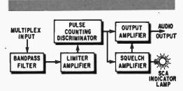
Fig. 3. Block diagram of the music adapter reveals unusual pulse counting discriminator used in missile radar telemetering systems.
