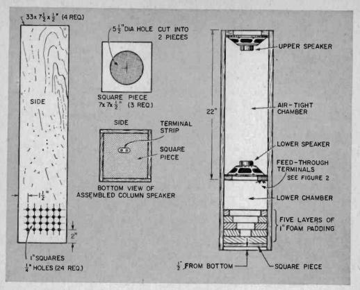
Column speaker can be assembled by fol- Wiring details for the column speaker are lowing construction details shown above. Construction can be speeded up by having lumber dealer cut plywood to exact sizes.
