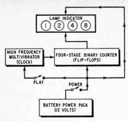
The Digilette simplified block diagram showing the four basic computer elements.
