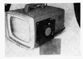
An aluminum grille panel cut to size mounts directly over the "Whisper Fan" input port to prevent accidental injuries and sucking up large particles and papers into the TV cabinet.
