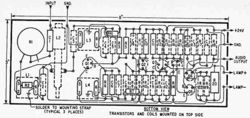
Fig. 5. Detail layout of parts on circuit board. Dashed lines indicate parts under board.
