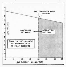
Exactly what ELVIS can put out is shown in volt-current graph with R4 fully CW.
